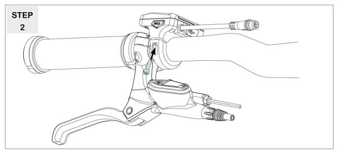
Mount and fasten the hex socket head screw with torque to 0.25 Nm (2.5 kgf/cm).
