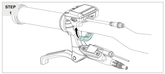
Mount the HMI hook on the handlebar.
